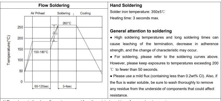
1) Time shown in the above figures is measured from the point when chip surface reaches temperature.
